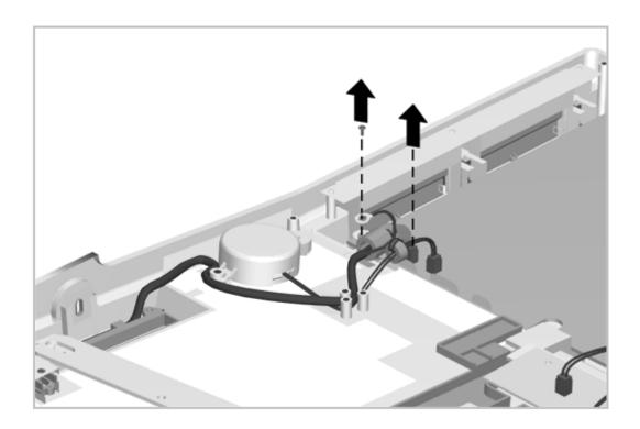
Figure 6-24. Disconnecting the Power Switch Board
